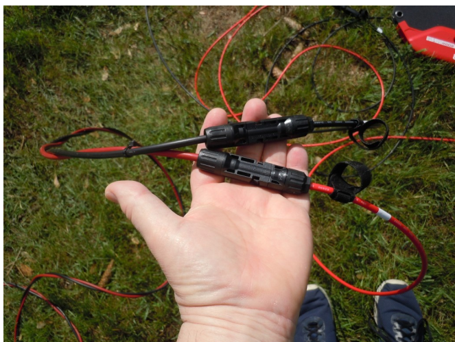
Figure 9: Connecting panels to extension
