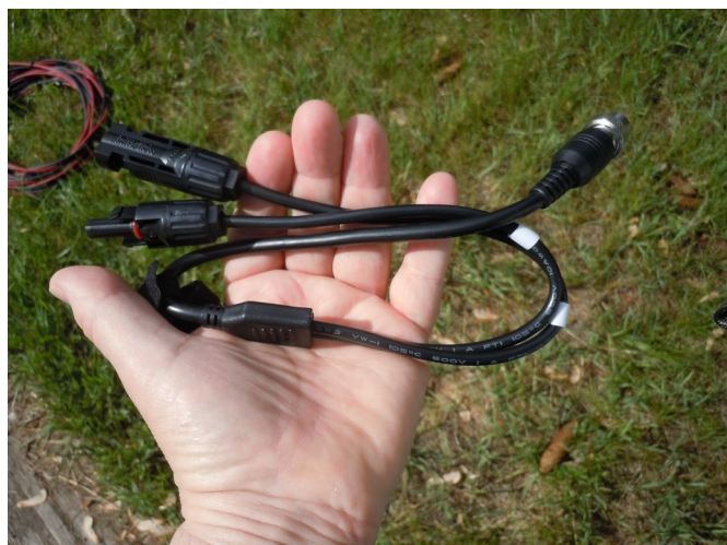
Figure 3: MC4 to GX16 adapter from Pecron
